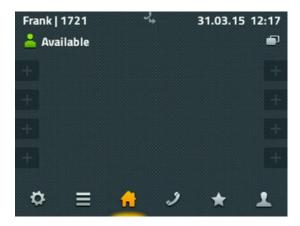
Your Presence is shown at the top left. To see a selection of various possibilities briefly press the icon. You can change your activity and add a note. The option "Do not disturb" can also be set: this usually turns off the ringing. The exact function of "Do not disturb" is determined in the account settings.
