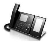
Separate installation is not necessary. Once plugged in, the extension module is ready for use immediately. Two apps are available on the extension module: the Home app with two pages and 16 freely programmable function keys as well as the Favorites app. Under settings, favorites, display, you can specify which favorite list should be displayed on which device. The functionality of the apps on the extension module correspond with those of the apps on the phone.
