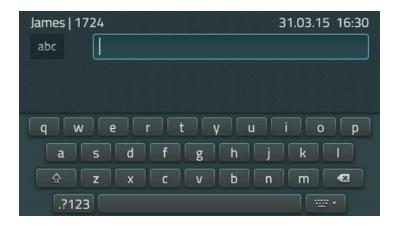
On the IP232 phone, the screen also displays a keyboard. Press on the input box to display the keyboard. Press the key at the bottom right-hand side next to the space bar for the keyboard to disappear.
